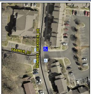
**ROMARE BEARDEN DR** Street 1 Name Stop Condition-Street 2 None Street 2 Name **FARMER ST** Stop Condition-Street 1 StopSign Possible Solutions: Remove & Replace Curb Ramp With **Two New Directional Ramps or** Equivalent. Surveyor Notes: N/A PROW/ADA: Not Found, R304.5.1, R304.5.3
