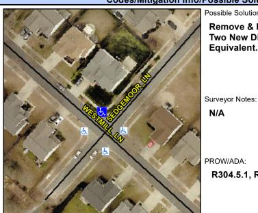
Street 1 Name Stop Condition-Street 2 Street 2 Name Stop Condition-Street 1 SEDGEMOOR LN None **WESTMILL LN**  Possible Solutions: **Remove & Replace Curb Ramp With Two New Directional Ramps or** Equivalent.
