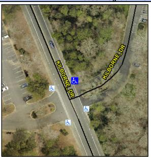
Street 1 Name Stop Condition-Street 2 Street 2 Name Stop Condition-Street 1 KILBORNE DR None **KILBORNE DR** None Possible Solutions: Remove & Replace Curb Ramp With Two New Directional Ramps or Equivalent. Surveyor Notes: N/A PROW/ADA: R304.2.2, R304.5.3
