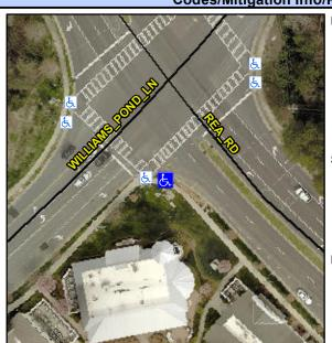
**REA RD** Street 1 Name Stop Condition-Street 2 Signal Street 2 Name N/A Stop Condition-Street 1 N/A Possible Solutions: Remove & Replace Entire Ramp. Restripe Crosswalk. Surveyor Notes: N/A PROW/ADA: Not Found, R304.5.1, R304.2.2
