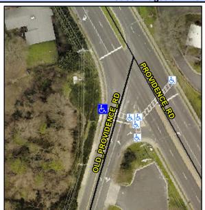
**OLD PROVIDENCE RD** Street 1 Name Stop Condition-Street 2 Signal Street 2 Name N/A Stop Condition-Street 1 N/A Possible Solutions: Remove & Replace Entire Ramp. Surveyor Notes: N/A PROW/ADA: Not Found, R304.2.2, R304.5.3
