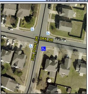
Street 1 Name OAK DR Stop Condition-Street 2 None **FOX POINT DR** Street 2 Name Stop Condition-Street 1 StopSign Possible Solutions: Remove & Replace Curb Ramp With Two New Directional Ramps or Equivalent. Surveyor Notes: N/A PROW/ADA: R304.5.1, R302.7
