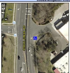
Street 1 Name Stop Condition-Street 2 Street 2 Name Stop Condition-Street 1 **ENTRANCE** None None Possible Solutions: **Remove & Replace Curb Ramp With** Two New Directional Ramps or Equivalent. Surveyor Notes:
