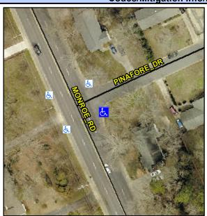
Street 1 Name Stop Condition-Street 2 Street 2 Name Stop Condition-Street 1 **PINAFORE DR** StopSign MONROE RD None Possible Solutions: Remove & Replace Curb Ramp With **Two New Directional Ramps or** Equivalent. Surveyor Notes: N/A PROW/ADA: Not Found, R304.2.2
