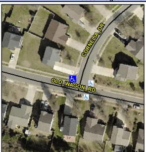
**OLD WAGON RD** Street 1 Name Stop Condition-Street 2 None **CORNELIA DR** Street 2 Name Stop Condition-Street 1 StopSign Possible Solutions: Remove & Replace Curb Ramp With Two New Directional Ramps or Equivalent. Surveyor Notes: N/A PROW/ADA: R304.5.1, R304.2.2
