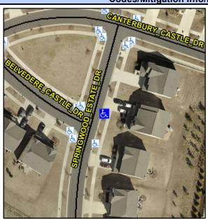
**SPRINGWOOD ESTATE DR** Street 1 Name Stop Condition-Street 1 None N/A Street 2 Name Stop Condition-Street 2 N/A Possible Solutions: Remove & Replace Curb Ramp With Two New Directional Ramps or Equivalent. Surveyor Notes: N/A PROW/ADA: Not Found, R304.5.3
