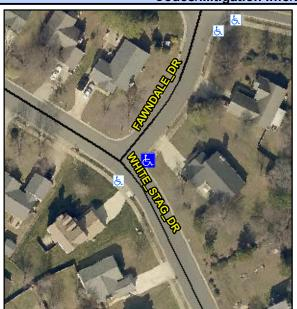
WHITE STAG DR Street 1 Name Stop Condition-Street 2 None Street 2 Name N/A Stop Condition-Street 1 N/A Possible Solutions: Remove & Replace Entire Ramp. Remove & Replace Gutter. Surveyor Notes: N/A PROW/ADA: Not Found, R304.5.1, R304.5.3, R304.2.3, R305.1.4, R305.2, R304.5.4
