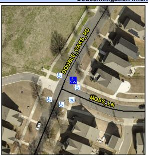
**DOUBLE OAKS RD** Street 1 Name Stop Condition-Street 1 None Street 2 Name N/A Stop Condition-Street 2 N/A Possible Solutions: Remove & Replace Entire Ramp. Surveyor Notes: **GAP IN LNDG WITH GRAVEL** PROW/ADA: R304.2.2, R302.7
