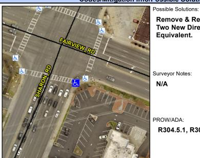
**SHARON RD** Street 1 Name Stop Condition-Street 1 Signal Street 2 Name N/A Stop Condition-Street 2 N/A Remove & Replace Curb Ramp With Two New Directional Ramps or Equivalent.
