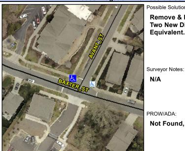
**BAXTER ST** Street 1 Name Stop Condition-Street 2 Street 2 Name **AVANT ST** Stop Condition-Street 1 StopSign Remove & Replace Curb Ramp With **Two New Directional Ramps or** Equivalent.
