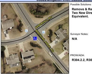
WINTHORP RIDGE RD Street 1 Name Stop Condition-Street 2 StopSign Street 2 Name **ARBORHILL RD** Stop Condition-Street 1 StopSign Remove & Replace Curb Ramp With **Two New Directional Ramps or** Equivalent.
