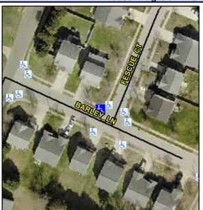
**BARLEY LN** Street 1 Name Stop Condition-Street 2 None Street 2 Name N/A Stop Condition-Street 1 N/A Possible Solutions: Remove & Replace Entire Ramp. Remove & Replace Gutter. Surveyor Notes: N/A PROW/ADA: Not Found, R304.5.3, R304.2.1, R304.5.4
