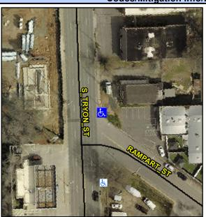
**S TRYON ST** Street 1 Name Stop Condition-Street 2 RAMPART ST Street 2 Name Stop Condition-Street 1 StopSign Possible Solutions: Remove & Replace Curb Ramp With Two New Directional Ramps or Equivalent. Surveyor Notes: N/A PROW/ADA: Not Found, R304.5.1, R304.2.2
