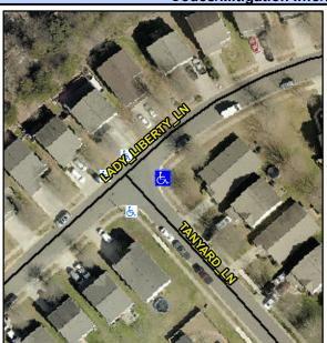
LADY LIBERTY LN Street 1 Name Stop Condition-Street 2 **TANYARD LN** Street 2 Name Stop Condition-Street 1 StopSign Possible Solutions: Remove & Replace Curb Ramp With Two New Directional Ramps or Equivalent. Surveyor Notes: N/A PROW/ADA: Not Found, R304.5.1, R304.5.3
