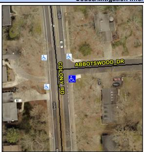
Stop Condition-Street 1 Street 2 Name Stop Condition-Street 2 **Remove & Replace Curb Ramp With** Two New Directional Ramps or Equivalent.
