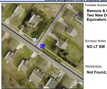
**ALTLIFF CT** Street 1 Name Stop Condition-Street 1 StopSign Street 2 Name N/A Stop Condition-Street 2 N/A Possible Solutions: Remove & Replace Curb Ramp With Two New Directional Ramps or Equivalent.
