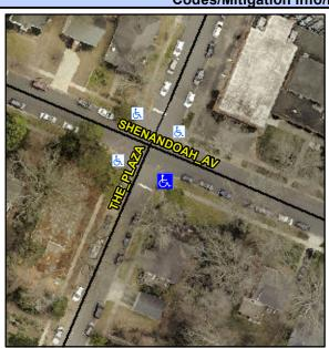
SHENANDOAH AV Street 1 Name Stop Condition-Street 2 THE PLAZA Street 2 Name Stop Condition-Street 1 StopSign Possible Solutions: Remove & Replace Curb Ramp With Two New Directional Ramps or Equivalent. Surveyor Notes: N/A PROW/ADA: Not Found, R304.2.2, R304.5.3
