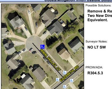
**IRWIN VALLEY CT** Street 1 Name Stop Condition-Street 1 None Street 2 Name N/A Stop Condition-Street 2 N/A Remove & Replace Curb Ramp With **Two New Directional Ramps or** Equivalent.
