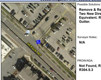
**ENTRANCE** Street 1 Name Stop Condition-Street 1 StopSign Street 2 Name N/A Stop Condition-Street 2 N/A Remove & Replace Curb Ramp With Two New Directional Ramps or Equivalent. Remove & Replace Gutter.
