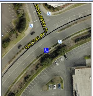
J W CLAY BV Street 1 Name Stop Condition-Street 2 None Street 2 Name N/A Stop Condition-Street 1 N/A Possible Solutions: Remove & Replace Entire Ramp. Surveyor Notes: N/A PROW/ADA: R304.5.1
