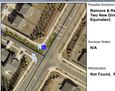
**SMITH RD** Street 1 Name Stop Condition-Street 1 None N/A Street 2 Name Stop Condition-Street 2 N/A Remove & Replace Curb Ramp With Two New Directional Ramps or Equivalent.
