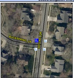
**BUCKSPRING LN** Street 1 Name Stop Condition-Street 2 StopSign Street 2 Name **SKYLINE DR** Stop Condition-Street 1 None Possible Solutions: Remove & Replace Curb Ramp With Two New Directional Ramps or Equivalent. Surveyor Notes: N/A PROW/ADA: R304.5.1, R304.5.3
