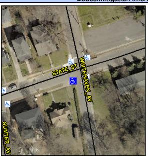
WHITEHAVEN AV Street 1 Name Stop Condition-Street 2 StopSign Street 2 Name STATE ST Stop Condition-Street 1 None Possible Solutions: Remove & Replace Curb Ramp With **Two New Directional Ramps or** Equivalent. Surveyor Notes: N/A PROW/ADA: Not Found, R304.5.1, R304.5.3
