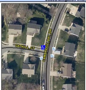
**GASKILL CT** Street 1 Name Stop Condition-Street 2 StopSign **CAMBRIDGE BAY DR** Street 2 Name Stop Condition-Street 1 None Possible Solutions: **Remove & Replace Curb Ramp With Two New Directional Ramps or** Equivalent. Surveyor Notes: N/A PROW/ADA: R304.5.1
