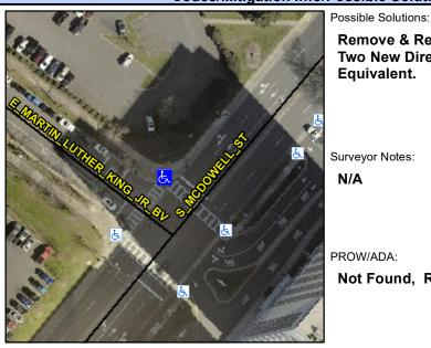
E MARTIN LUTHER KING JR BV Street 1 Name Stop Condition-Street 2 Signal Street 2 Name **S MCDOWELL ST** Stop Condition-Street 1 Signal Remove & Replace Curb Ramp With Two New Directional Ramps or Equivalent.
