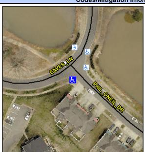
Street 1 Name Stop Condition-Street 2 Street 2 Name Stop Condition-Street 1 **PHIL ONEIL DR** StopSign **EAVES LN** None Possible Solutions: Remove & Replace Curb Ramp With **Two New Directional Ramps or** Equivalent. Surveyor Notes: N/A PROW/ADA: R304.5.1, R304.2.2
