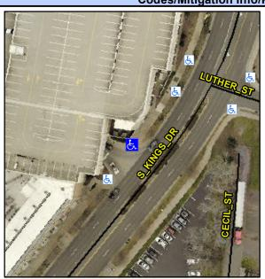
**ENTRANCE** Street 1 Name Stop Condition-Street 2 StopSign Street 2 Name **S KINGS DR** Stop Condition-Street 1 None Possible Solutions: Remove & Replace Curb Ramp With **Two New Directional Ramps or** Equivalent. Surveyor Notes: N/A PROW/ADA: Not Found, R304.2.2, R304.5.3
