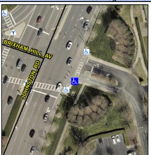
**BRIXHAM MILL AV** Street 1 Name Stop Condition-Street 1 Signal Street 2 Name N/A Stop Condition-Street 2 N/A Possible Solutions: Remove & Replace Entire Ramp. Surveyor Notes: N/A PROW/ADA: R304.5.1, R304.3.2
