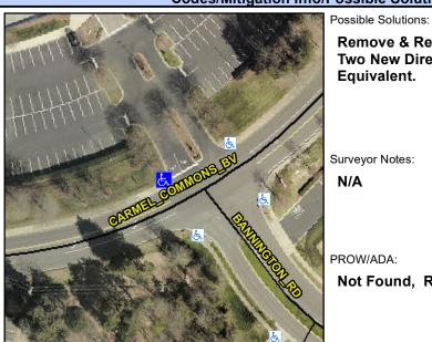
**CARMEL COMMONS BV** Street 1 Name Stop Condition-Street 2 None Street 2 Name **BANNINGTON RD** Stop Condition-Street 1 StopSign Remove & Replace Curb Ramp With Two New Directional Ramps or Equivalent.
