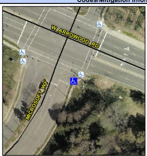
MICROSOFT WY Street 1 Name Stop Condition-Street 2 Signal Street 2 Name N/A Stop Condition-Street 1 N/A Possible Solutions: Remove & Replace Entire Ramp. Remove & Replace Gutter. Surveyor Notes: N/A PROW/ADA: R304.2.1, R304.2.2-Perp, R304.3.2-Para, R305, R302.7, R302.7.2,
