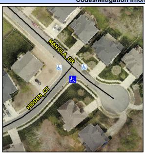
Street 1 Name Stop Condition-Street 2 Street 2 Name Stop Condition-Street 1 **MANGLA DR** None **HIDDEN CT** StopSign Possible Solutions: Remove & Replace Curb Ramp With Two New Directional Ramps or Equivalent.
