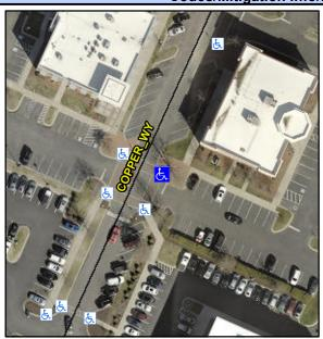
**COPPER WY** Street 1 Name Stop Condition-Street 1 None N/A Street 2 Name Stop Condition-Street 2 StopSign Possible Solutions: Compliance Description Remove & Replace Curb Ramp With Two New Directional Ramps or Equivalent. Surveyor Notes: N/A PROW/ADA: Not Found, R304.5.1
