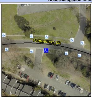
**FARMHURST DR** Street 1 Name Stop Condition-Street 2 None **ENTRANCE** Street 2 Name Stop Condition-Street 1 None Possible Solutions: Remove & Replace Curb Ramp With Two New Directional Ramps or Equivalent. Surveyor Notes: N/A PROW/ADA: R304.5.3
