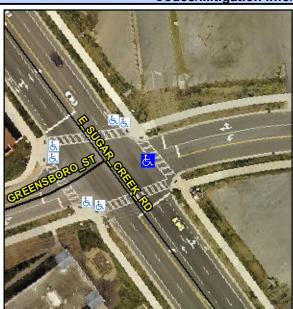
**GREENSBORO** Street 1 Name Stop Condition-Street 2 Signal **E SUGAR CREEK** Street 2 Name Stop Condition-Street 1 Signal Possible Solutions: Remove & Replace Curb Ramp With **Two New Directional Ramps or** Equivalent. Surveyor Notes: N/A PROW/ADA: Not Found, R304.5.3
