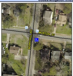
Street 1 Name StopSign Stop Condition-Street 1 MORTON ST Street 2 Name N/A Stop Condition-Street 2 N/A Possible Solutions: Remove & Replace Entire Ramp. Surveyor Notes: LT RP < 5% PROW/ADA: Not Found, R304.5.1, R304.5.1, R304.5.3
