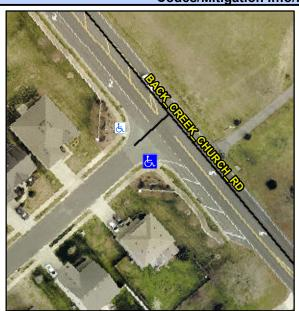
**BELMONT RUN LN** Street 1 Name Stop Condition-Street 2 StopSign Street 2 Name N/A Stop Condition-Street 1 N/A Possible Solutions: Remove & Replace Entire Ramp. Remove & Replace Gutter. Surveyor Notes: N/A PROW/ADA: Not Found, R305.2, R302.7.2, R304.5.4, R304.5.3
