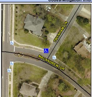
Stop Condition-Street 2 Street 2 Name Stop Condition-Street 1 Possible Solutions: Remove & Replace Curb Ramp With Two New Directional Ramps or Equivalent. Surveyor Notes: N/A
