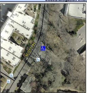
SCOTT AV Street 1 Name Stop Condition-Street 2 None Street 2 Name **LOOP RD** Stop Condition-Street 1 StopSign Possible Solutions: Remove & Replace Curb Ramp With Two New Directional Ramps or Equivalent. Restripe Crosswalk. Surveyor Notes: N/A PROW/ADA: Not Found, R304.2.2, R304.5.3
