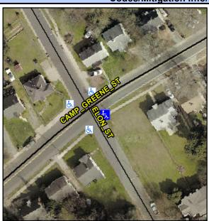
**CAMP GREENE ST** Street 1 Name Stop Condition-Street 2 None **ELON ST** Street 2 Name Stop Condition-Street 1 StopSign Possible Solutions: Remove & Replace Curb Ramp With Two New Directional Ramps or Equivalent. Surveyor Notes: N/A PROW/ADA: R304.2.2
