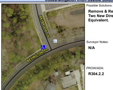
Street 1 Name Stop Condition-Street 2 Street 2 Name Stop Condition-Street 1 **BEVINGTON PL** None **BAYBROOK LN** StopSign Remove & Replace Curb Ramp With **Two New Directional Ramps or**
