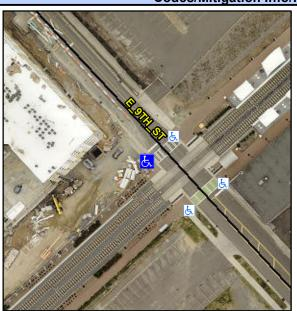
Street 1 Name E 9TH ST Stop Condition-Street 1 None Street 2 Name N/A Stop Condition-Street 2 N/A Possible Solutions: Remove & Replace Curb Slope and Extend Ramp. Surveyor Notes: N/A PROW/ADA: **Not Found**
