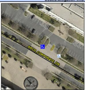
ARCO CORPORATE DR Street 1 Name Stop Condition-Street 2 None Street 2 Name **ENTRANCE** Stop Condition-Street 1 None Possible Solutions: Remove & Replace Curb Ramp With Two New Directional Ramps or Equivalent. Surveyor Notes: N/A PROW/ADA: R304.5.1, R304.2.2
