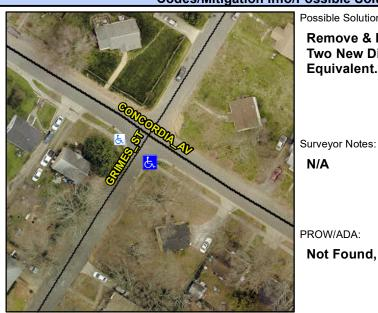
**GRIMES ST** Street 1 Name Stop Condition-Street 1 StopSign Street 2 Name N/A Stop Condition-Street 2 N/A Possible Solutions: **Remove & Replace Curb Ramp With** Two New Directional Ramps or Equivalent.
