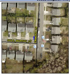
**GOLD WORTHY CT** Street 1 Name Stop Condition-Street 2 StopSign Street 2 Name **EMMONS LN** Stop Condition-Street 1 None Possible Solutions: Remove & Replace Curb Ramp With **Two New Directional Ramps or** Equivalent. Surveyor Notes: N/A PROW/ADA: Not Found, R304.5.3
