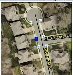
**OPEN BOOK LN** Street 1 Name Stop Condition-Street 1 None N/A Street 2 Name Stop Condition-Street 2 N/A Possible Solutions: Remove & Replace Curb Ramp With Two New Directional Ramps or Equivalent. Surveyor Notes: N/A PROW/ADA: Not Found, R304.5.1
