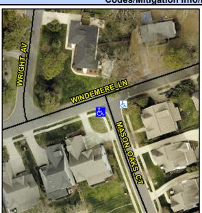
**MASON OAKS CT** Street 1 Name Stop Condition-Street 1 StopSign Street 2 Name N/A Stop Condition-Street 2 N/A Possible Solutions: **Remove & Replace Curb Ramp With Two New Directional Ramps or** Equivalent. Surveyor Notes:
